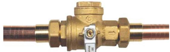
*Filterball with Male Union ends. Solder Unions and flat washer secure copper pipes. No need to spring pipes apart. Flat faced connections also suitable for Press-Fit, Friatherm, Unipipe etc. Note thread is one size larger than nom. valve size. (Please check lead-time on this version).*
