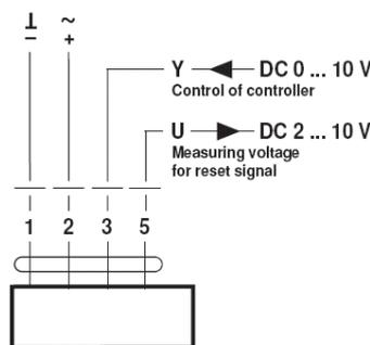
**Override control (frost protection circuit)**
