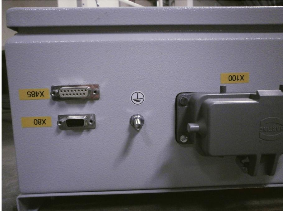
This connector provides the Temperature sensor FLOW MREF to the MRI.
