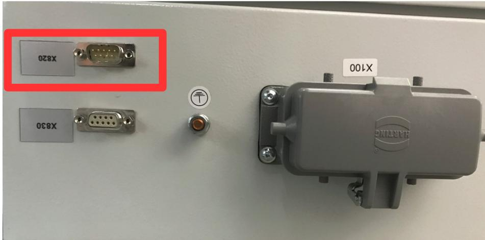
A removed or non working CAN-Bus will result in a permanent Nightmode sequence.
