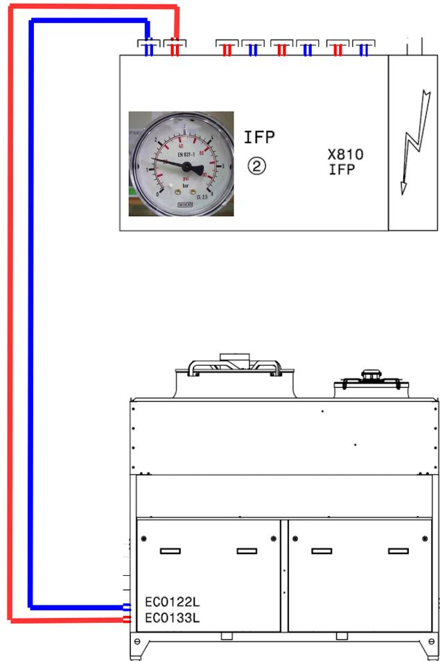
A installed and working automatic Airvent in supply & return piping with a correct static pressure will determin most of the failures and is recommended for this system.
