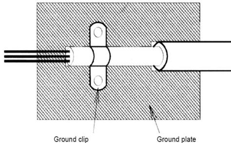
Moreover, cable shields must be connected with purpose-made ground clips.
