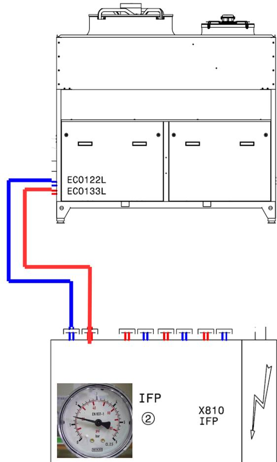
A installed and working automatic Airvent in supply&return piping with a correct static pressure will determin most of the failures and is recommended for this system.
