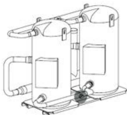
Figure 140: Example Compressor assembly – oil sight glass
