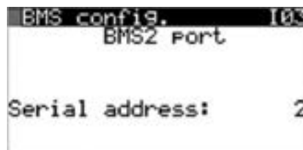
Figure 91: Configuring a unit as a slave - Serial address
