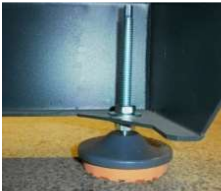
Figure 7: Machine base (foot) - mounting on the baseplate
