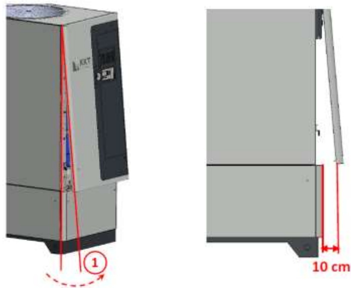
Figure 2: Demounting the side panel of the switch cabinet
