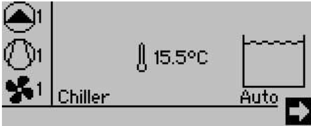
Figure 20: Start screen with tank and without alarm
